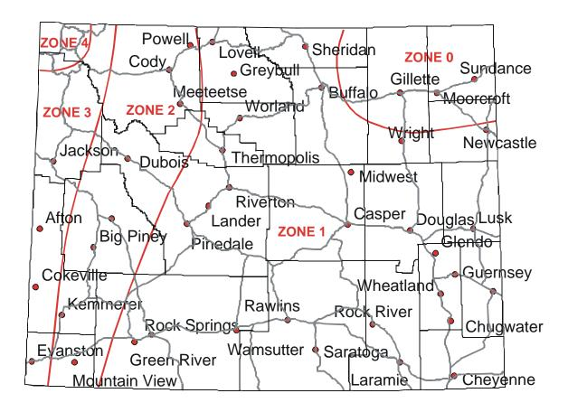
Figure 1. UBC Seismic Zone Map.
