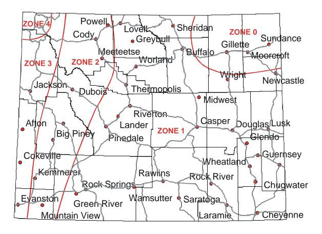
Figure 1. UBC Seismic Zone Map.
