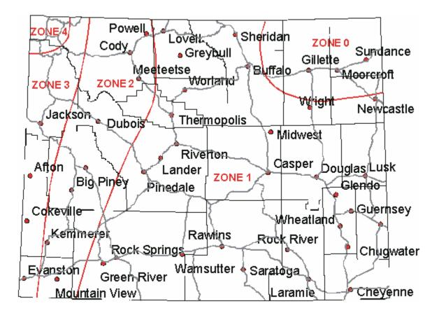
Figure 1. UBC Seismic Zone Map.
